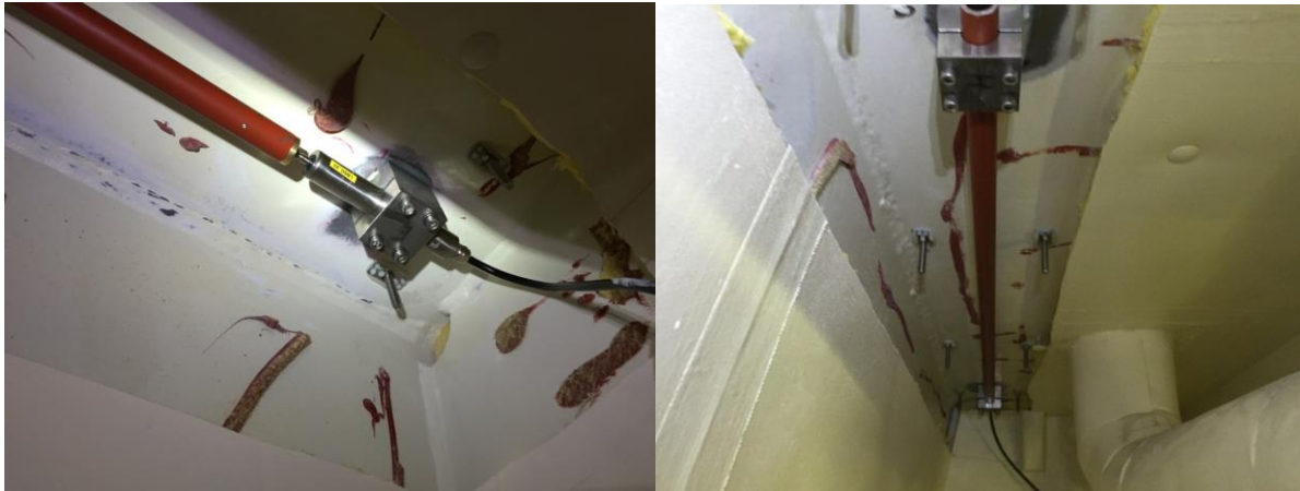
Figure 5: Pictures of long base strain gauges on board USCGC STRATTON
